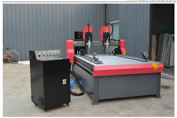
Rotary Axis CNC Router Machine is the other type of 4 axis CNC router. Except for carving, cutting, drilling, pocketing, routing, and other functions that a 3 axis router machine can achieve, it is also good at making cylindrical parts. For example, wood table and chair legs, wood handrails, wood or plaster building columns, 3D statues of wood, rubber, foam, etc.
