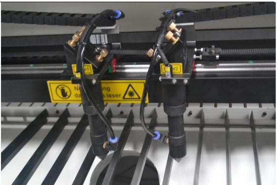
High working efficiency double laser head with red light positioning system,imported lens which will make the light beam stable and powerful.
