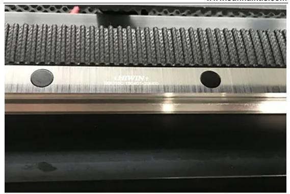
Adopted Taiwan HIWIN linear guide rail, fast running and high positioning accuracy for a longer time, improves the accuracy of engraving and cutting.
