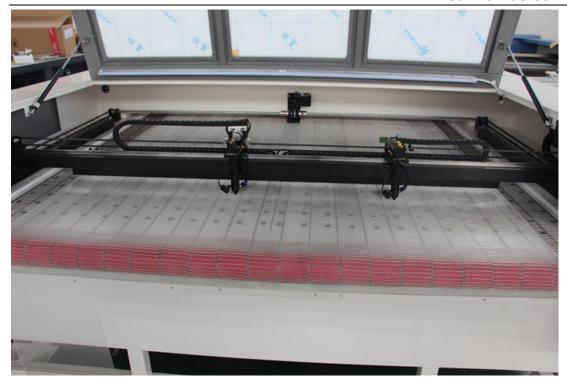
High quality duble laser head with red light positioning system,imported lens which will make the light beam stable and powerful. Air-cooled system to protect the lens and laser head.
