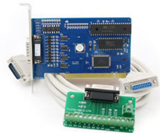
NC-studio Control system
